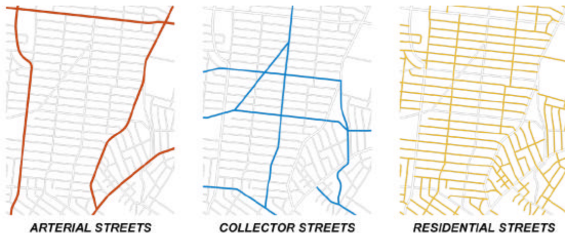
Figure 2.2.1. Functional Classification of Southampton Roadways
