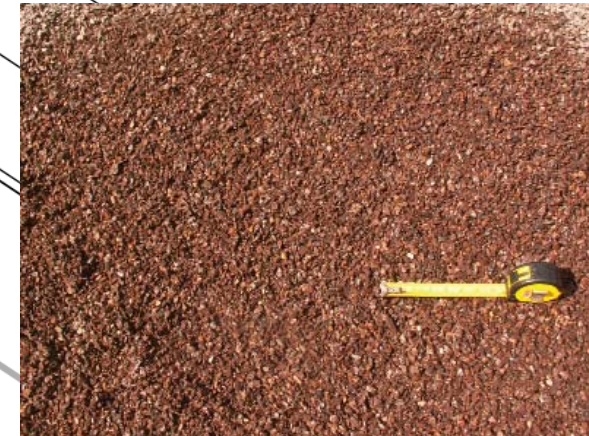
TRAP CHIP GRAVEL PAVING
